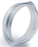
Mounting frame for ceiling thickness from 10 to 30 mm / 0.39" to 1.18"
